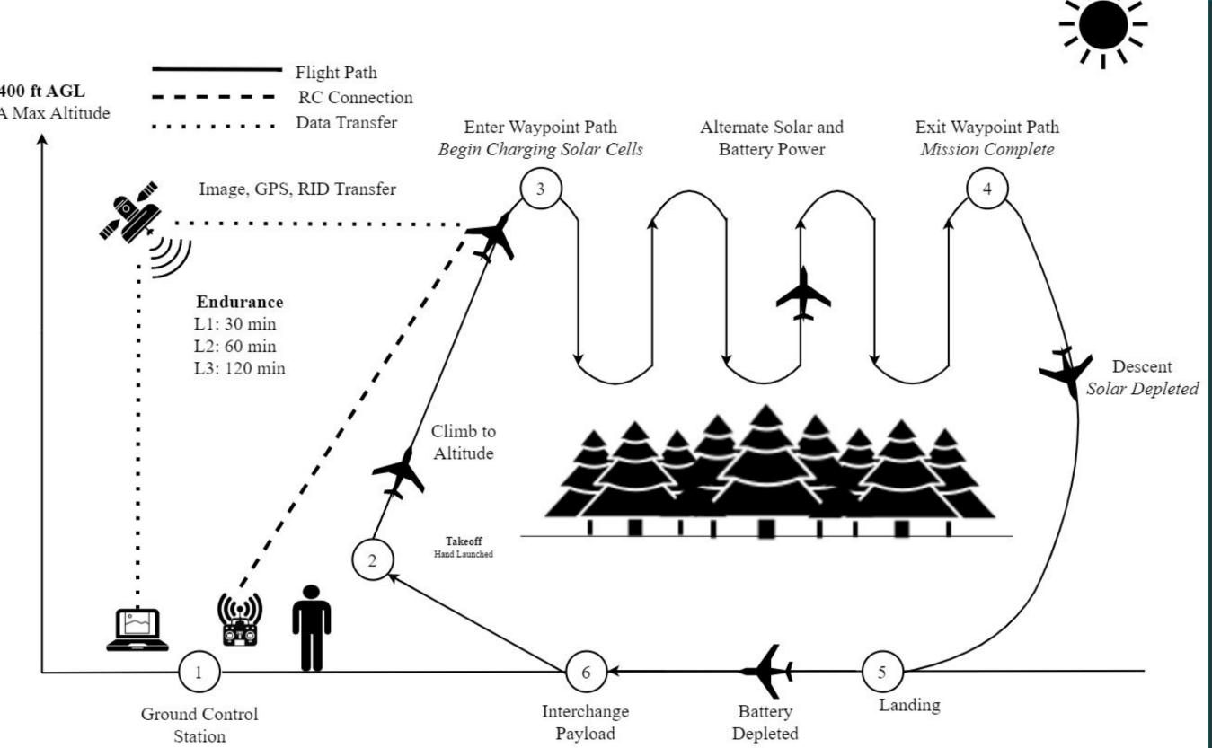
The L.O.R.A.X. UAV was designed to provide the NC forest service with a cost-effective method of aerial surveillance. It is hand launched to allow for operations in remote areas and is equipped with a flight controller for autonomous missions. Solar panels are used to extend the UAV's range and endurance. If the battery is depleted or if the mission is accomplished the UAV can make a belly landing to swap batteries or payload sensors.
