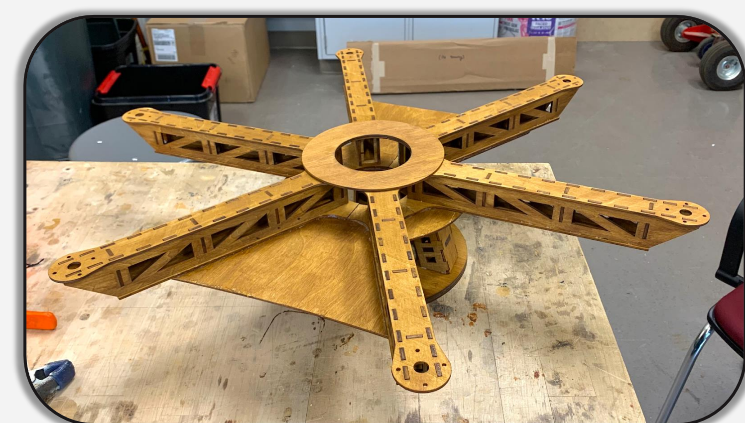
Laser Cut Basswood Sealed and Glued Together
