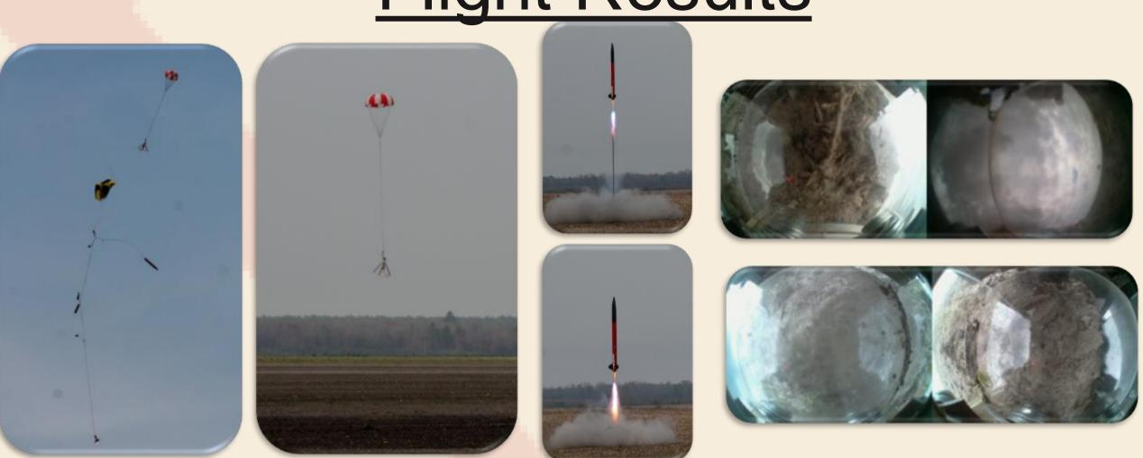
The team conducted test flights on February 20th and March 27th, 2021 and a final flight on April 10th, 2021. During the Payload Demonstration Flight, LOPSIDED was successfully jettisoned from the launch vehicle. On the final flight, LOPSIDED successfully captured images using the POS after landing. The highest altitude the Launch Vehicle reached was 3,084 ft. The Launch Vehicle's recovery system performed nominally.
