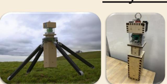
**Top Section**: contains the POS cameras and recovery hardware.
