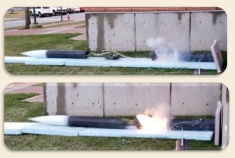
A new calculator for sizing black powder ejection charges using 4F black powder was developed to adapt to issues encountered in previous years. Online calculators used in the past by previous teams had been found to generally underestimate the charge size needed for a given chamber volume
