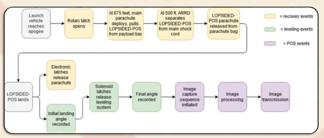
The payload consists of two main systems – the Lander for the Observation of Planetary Surface Inclination, Details, and Environment Data (LOPSIDED), and the Planetary Observation System (POS). LOPSIDED is a planetary lander that houses the POS, which is used to deliver data in the form of images captured from LOPSIDED's landing site.
