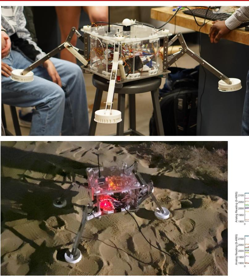
For the CRIA prototype, the camera gimbal was tested by shining a light source in the view of the camera while a Simulink tracking model was running. The camera is capable of viewing IR light, meaning that in a permanently-shadowed crater an IR emitter on LLAMA can be tracked. CRIA's ability to communicate with LLAMA via a radio transceiver was also successfully tested
