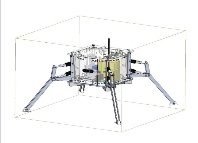
The control system consists of a Raspberry Pi 4B and 3 Adafruit DC & Stepper Motor Bonnets, an Arduino for reading the 12 potentiometers/joint angles, and an IMU for orientation feedback. Additionally, a radio transceiver is mounted to the top for communications and an IR camera is mounted to the front for hazard detection. The power system consists of a 5V battery pack for the Raspberry Pi and an 14.8V lithium-ion battery pack regulated to 12V to power our 8 linear actuators and 4 DC motors.
