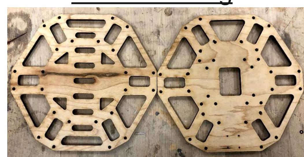
Laser cut plywood hub plates that provide the central structure of the aircraft
