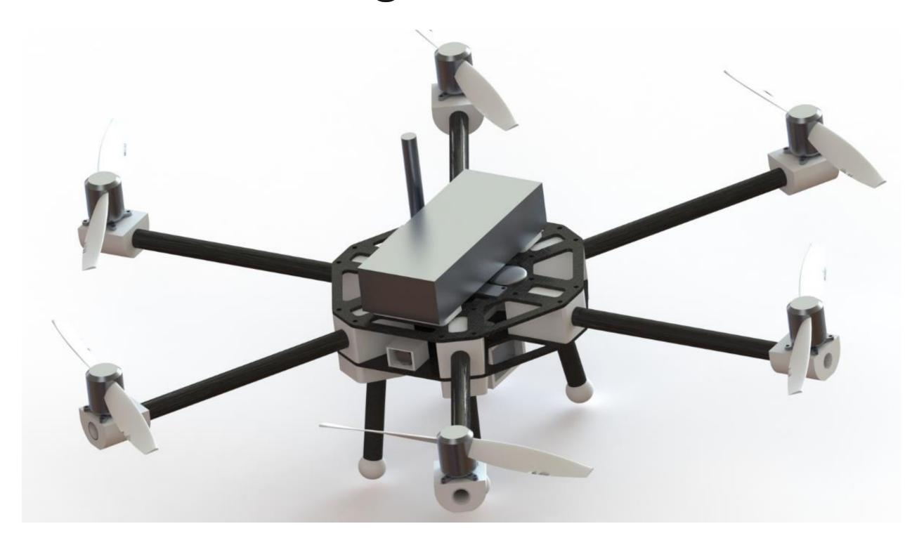
Six-rotored, semi-autonomous aerial vehicle equipped with a multispectral agricultural camera, an FPV camera, and a gas sensor
