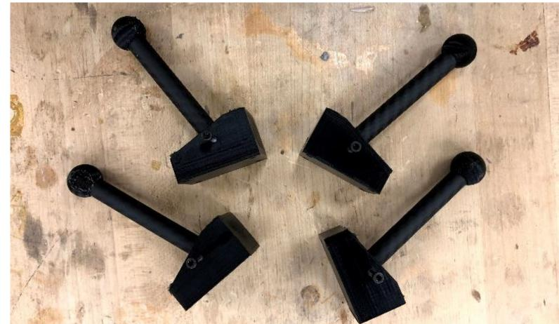
Landing gear consisting of 3D printed components and carbon fiber rods
