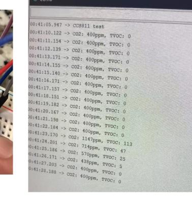
The two photos above on the right demonstrate the air quality sensing capabilities, including eCO2 and VOC levels
