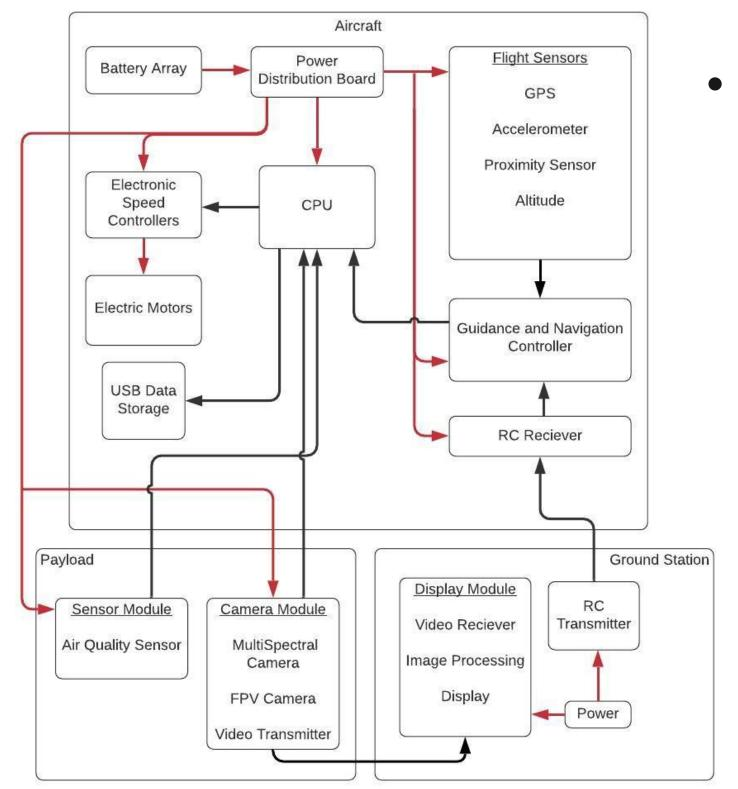
This diagram shows how power and data is distributed throughout the aircraft's subsystems
