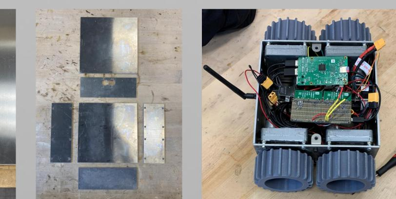
Interconnections between subsystem components were tested prior to installation for issues ensuring no faulty components were installed, with emphasis on the power system
