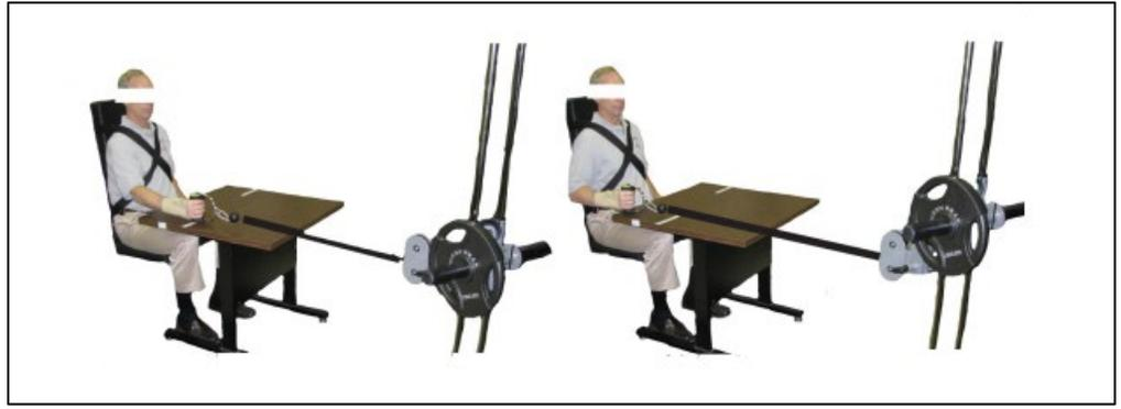
**Figure 3.** Example pulling task using Powertec system alone [48].
