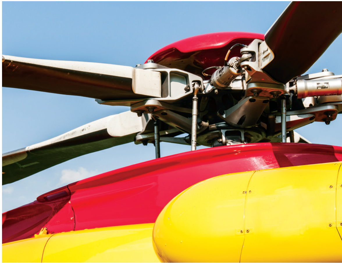
LORD dynamic components react loads and allow motion to enable helicopters to fly.
