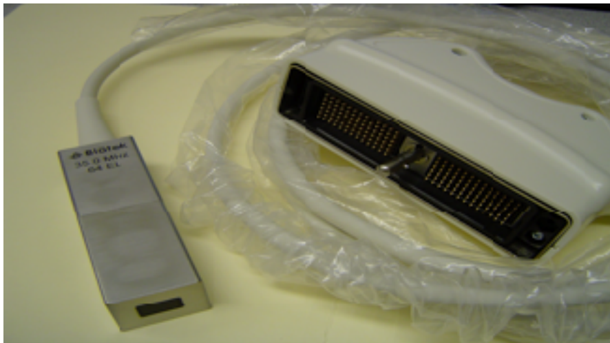
Figure 6. Photograph of a micromachined 35 MHz phased array (64-element).
