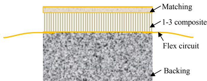
Figure 3. Schematic view of phased array acoustic stack.
