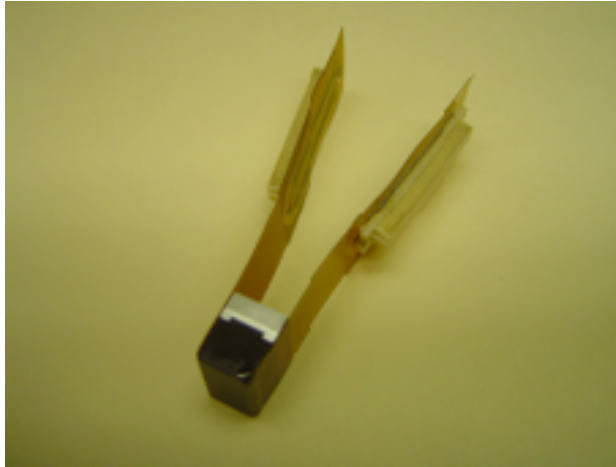
Figure 5. A 35 MHz 64-element PC-MUT phased array without housing and cable connection.
