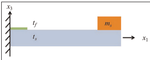
Figure 9. Schematic picture of a flexoelectric microaccelerometer.
