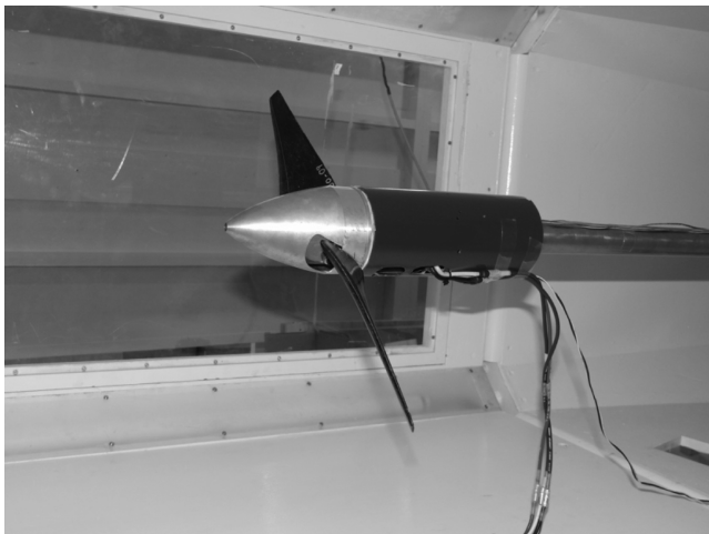
Fig. 20 8009 PVPP in the NCSU subsonic tunnel for testing.
