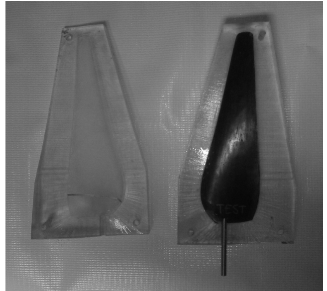
Fig. 18 Rapid prototyped molds with an example propeller blade.
